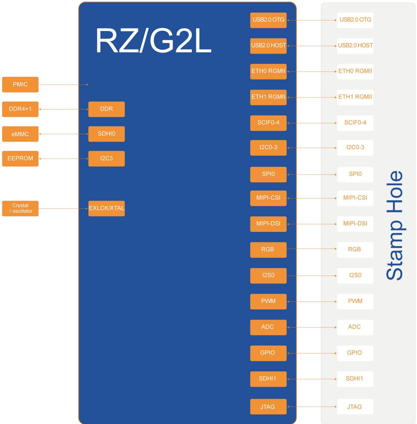
MYC-YG2LX CPU Module Function Block Diagram
