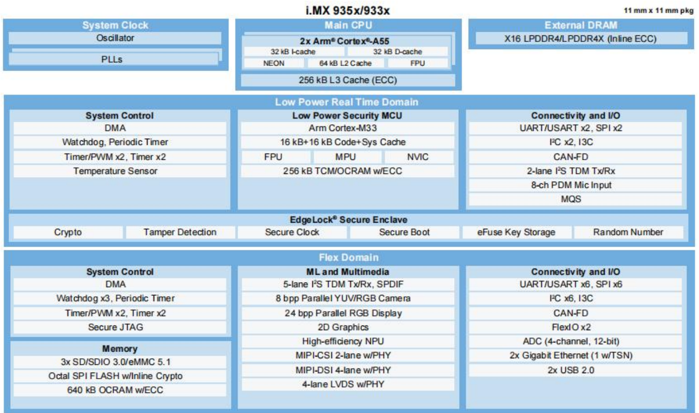
i.MX93 Processor Block Diagram
