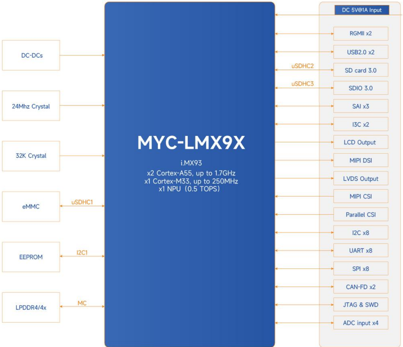
MYC-LMX9X Function Block Diagram
