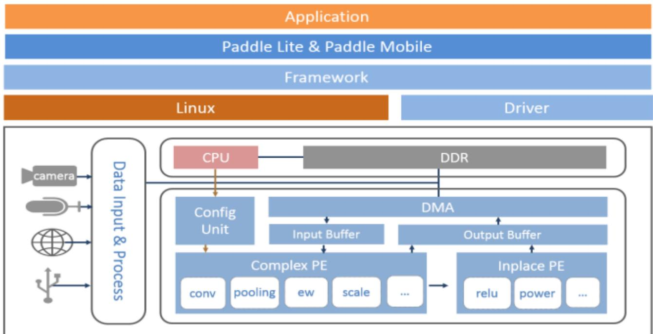
Figure 1-10 Software Architecture of FZ5 EdgeBoard AI Box
